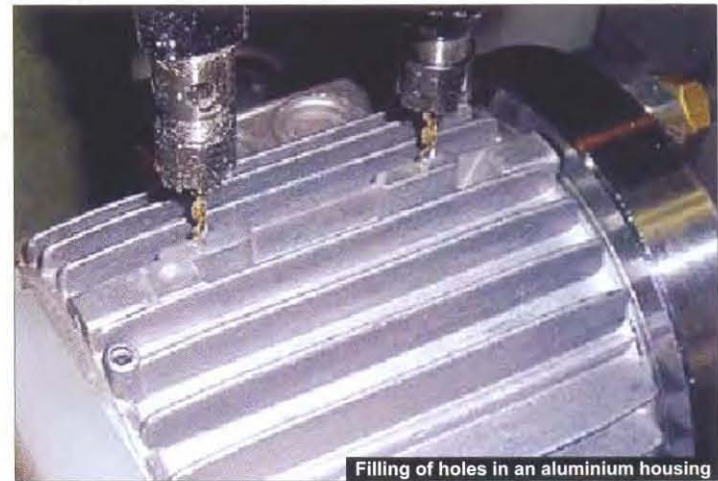
Filling of holes in an aluminium housing
