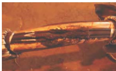
Filler damage, core intact
